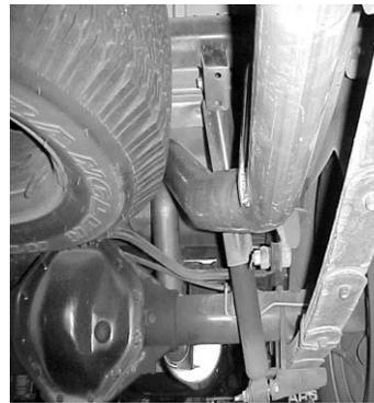
INSTALL OVERAXLE TAILPIPE #C AND CONNECT IT TO THE MUFFLER AND CLAMP DOWN USING HANGER #D. INSERT WELDED HANGER INTO RUBBER GROMMET. ROLL THE TAILPIPE UNTIL YOU FIND THE CORRECT ANGLE. THE SPARE TIRE ON SOME VEHICLES MAY NEED TO BE LOOSENED AND PUSHED TO THE DRIVER SIDE FOR CLEARANCE PURPOSES.
