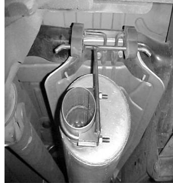
INSTALL MUFFLER # B ONTO HEADPIPE WITH INLET TOWARDS CONVERTER USING CLAMP #E. USE A JACK STAND TO SUPPORT THE MUFFLER. MAKE SURE THE MUFFLER IS LEVEL. THE OUTLET OF THE MUFFLER WILL BE AT ABOUT 7 TO 8 O'CLOCK. THE MUFFLER INLET WILL BE LOOKING INTO THE LOUVERS TOWARDS THE MOTOR. ATTACH HANGER #D TO OUTLET OF MUFFLER AND INSERT INTO WELDED HANGER.
