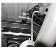
INSTALL HANGER #H AS PROVIDED. VERTICAL ROD ON HANGER #H SHOULD BE TO THE LEFT OF THE CENTER OF THE MUFFLER.
