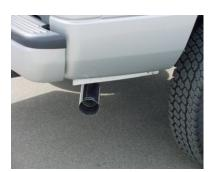
INSTALL STAINLESS STEEL TIP. CLAMP DOWN. WHEN YOU HAVE EVERYTHING IN PLACE, FIRMLY TIGHTEN ALL BOLTS AND CLAMP DOWN SECURELY. TO CLEAN STAINLESS STEEL TIP USE ANY STAINLESS STEEL OR ALUMINUM CLEANER.
