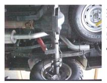
INSTALL THE OVERAXLE TAILPIPE #C TO THE MUFFLER AND CONNECT WITH CLAMP #F. BUT DO NOT TIGHTEN. SLIDE WELDED HANGERS INTO RUBBER GROMMETS.
