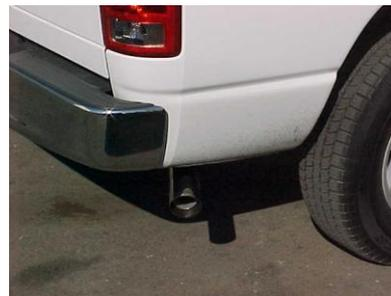
INSTALL STAINLESS STEEL TIP. WHEN YOU HAVE EVERYTHING IN PLACE, FIRMLY TIGHTEN ALL BOLTS AND CLAMP DOWN SECURELY. TO CLEAN STAINLESS STEEL TIP USE ANY STAINLESS STEEL CLEANER AND SCOTCH BRITE PAD.
