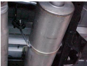
SLIDE BAND CLAMP #G ONTO MUFFLER WITH BOLT KIT # H. INSERT HANGERS INTO RUBBER GROMMETS.
