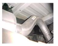
Install the over axle tailpipe # D into the muffler 1-1/2" to 2". Secure to the muffler using clamp # G. Do not tighten.
