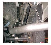
Install the exit pipe # E on to the tailpipe. Insert welded hanger into rubber grommet. Secure together with clamp # G. Do not tighten. Roll the exit pipe and tailpipe until it is at the correct angle for your truck with proper clearances.
