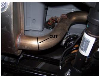
4. Install headpipe #A onto your existing stock front pipe and secure with clamp #F. Do not tighten.
