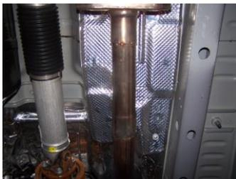
5. Install muffler #B onto headpipe 1 1/2-2". Use a jack stand to support the muffler. Use clamp #F to secure the muffler to the headpipe. Do not tighten. (Before installing tailpipes you must remove spare tire and heat shield.)
