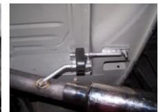
7. Install passenger side tailpipe #C into muffler 1.5-2". Use clamp #G to secure. Do not tighten. Insert welded hangers into rubber grommets.
