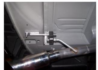
8. Install driver side over axle tailpipe #D into the muffler 1.5-2". Use clamp #G to secure. Do not tighten. Insert welded hanger into rubber grommet.
