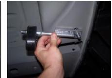
6. Install the rear hangers at the rear of the frame on both driver and passenger side. Slide bolt and tab into the frame as shown. Then attach the rear hanger with rubber grommet.
