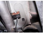
5. Install the overaxle tailpipe #C to the muffler 1.5"-2". Use clamp #E to secure tailpipe to muffler. Do not tighten. Now install your stock grommet on your rear hanger, and bolt it back onto the frame, using stock hardware.
