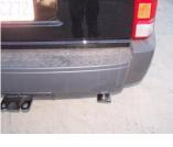
11. Install stainless steel tip. Clamp down. When you have everything in place, firmly tighten all bolts and clamps down securely. Use stainless steel cleaner and a Scotch Brite pad weekly to prevent tip from discoloration. Inspect all fasteners after 25-50 miles of operation and re-tighten as necessary.
