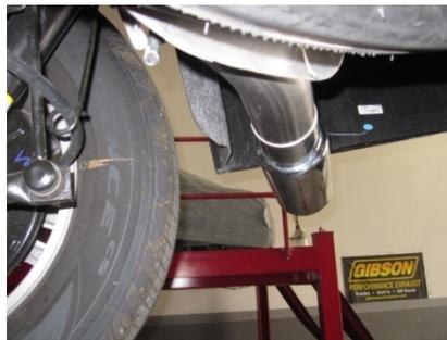
6. With proper clearance from spare tire install the exhaust tip onto the tailpipe. The system was designed to have the tip 1" below the quarter panel of the vehicle. With the tip in your desired position begin to tighten down all clamp connections from the
