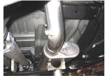
4. Install over axle pipe Item # C into the muffler outlet. Slip the hangers into the rubber grommets and keep tailpipe loose use clamp #E to secure together.
