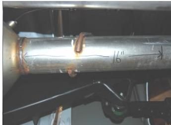
2. Short Beds: To remove your stock exhaust, Measure 16" from the end of the factory converter and Particular filter then cut. Do not damage your factory grommets. You will re-use them
