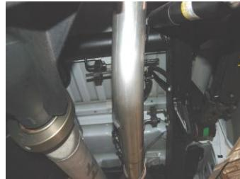
3. Slide the over axle tailpipe #A into the muffler 1.5"-2". Use clamp #C to secure tailpipe to the stock muffler. Do not tighten. Insert welded hanger into rubber grommet.
