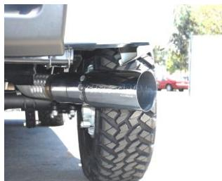
4. Next, slide exit pipe #B onto tailpipe. Use clamp #C to secure the exit pipe to the tailpipe. Do not tighten. Insert welded hangers into Rubber grommets
