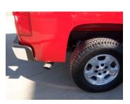
8. Install stainless steel tip. Clamp down. When you have everything in place, firmly tighten all bolts and clamps down securely. Use stainless steel or aluminum cleaner to polish tips. Inspect all fasteners after 25-50 miles of operation and re-tighten as necessary.
