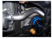
**4.** Install overaxle tailpipe #C into muffler.
