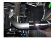
**5.** Use clamp #E to secure tailpipe to the muffler. DO NOT TIGHTEN.
