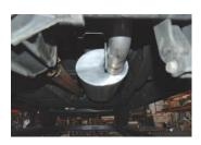
4. Install muffler #B onto headpipe #A 1½"-2" with the louvers facing towards the converter. Use a jack stand to support the muffler. Use clamp #E to secure the muffler to the headpipe. Do not tighten. Muffler inlet is looking into the louvers. Muffler outlet should be at the 3 o'clock position.
