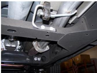
3. Install headpipe #A onto your existing stock flange and secure using the stock hardware. Do not tighten. Insert welded hanger into rubber grommet.
