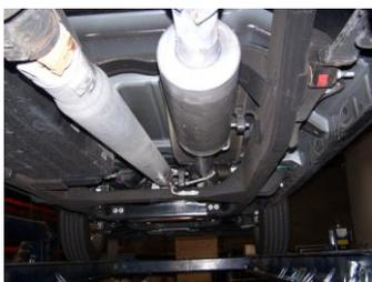
4. Install muffler #B onto headpipe 1½"-2" with the louvers facing towards the converter. Use a jack stand to support the muffler. Use clamp #F to secure the muffler to the headpipe. Do not tighten. Muffler inlet is looking into the louvers.
