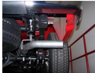
6. Slide exit pipe #D onto overaxle tailpipe using clamp #E to secure. Rotate exit pipe until it is at the correct angle for your truck. Insert welded hanger into rubber grommet.
