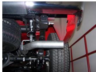
6. Slide exit pipe #D onto over axle tailpipe using clamp #E to secure. Rotate exit pipe until it is at the correct angle for your truck. Insert welded hanger into rubber grommet.
