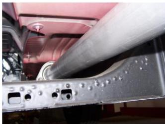
3. Bolt headpipe #A to the stock flange re-using the factory nuts and bolts. Insert welded hanger into rubber grommet. Do not tighten, just make snug.
