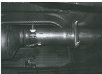
4. Slide the muffer into the headpipe at least 1.5"-2". Use a jack stand to support the muffer. Use clamp #E to secure muffer assembly to the headpipe. The outlet of the muffer will be at approximately 11 o'clock. The muffer inlet is looking into the louvers. Do not tighten.
