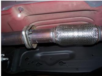
2. To remove stock exhaust, unbolt it at the flange behind the Y-pipe. Make sure to leave all rubber grommets in the factory location. You will re-use stock nuts and bolts. For easier removal of exhaust, cut behind the muffler. Use WD-40 to remove hangers from grommets.
