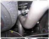
Install the over axle tailpipe #C into the muffler 1½-2". Secure to muffler using clamp #D. Insert welded hangers into rubber grommets. DO NOT TIGHTEN.
