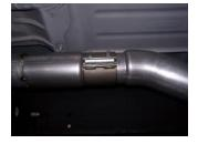
Install head pipe #A onto your factory down pipe using factory clamp to secure. DO NOT TIGHTEN. Insert welded hangers into rubber grommets.
