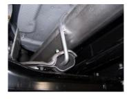
Install down pipe #A onto turbo and secure with factory clamp. DO NOT TIGHTEN. Insert welded hanger into bottom hole of rubber grommet.
