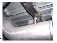
Install muffler #C onto head pipe 1½-2", with louvers facing forward. Use a jack stand to support the muffler. Use clamp #E to secure the muffler to the head pipe. Muffler inlet is looking into the louvers. DO NOT TIGHTEN.
