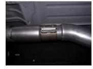
Install head pipe #B onto down pipe using factory clamp to secure. DO NOT TIGHTEN. Insert hangers into rubber grommets.
