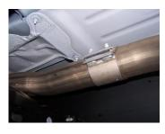
Lay out the exhaust on the floor so it looks like the drawing and compare parts with manual. To remove the stock exhaust unclamp it just in front of muffler. Save factory clamp. Leave all rubber grommets in place. Use WD-40 to aid in removal of exhaust and hangers.
