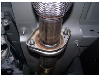
**1.** To remove the stock exhaust, remove it from the two bolt flange in front of the muffler. Do not throw away you will re-use bolts. Disengage the welded hangers using WD-40 from the OEM rubber grommets. Do not damage or remove the rubber grommets as you will reuse them to mount your new system. Now, cut off tailpipe before and after rear axle for removal.
