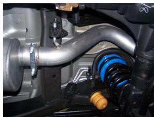
**4.** Install overaxle tailpipe #C into muffler. Insert welded hangers into rubber grommets.
