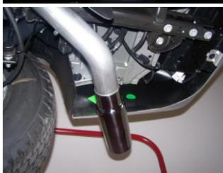
**3.** Install muffler #B onto head pipe #A 1 1/2"-2". Use a jack stand to support the muffler. Use clamp #E to secure the muffler to the headpipe. Do not tighten. Muffler outlet will be in the 11 o'clock position. Muffler inlet is looking into the louvers.
