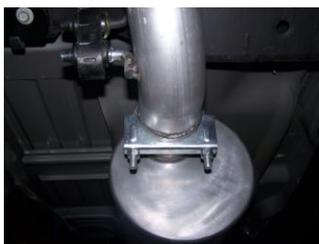
**6.** Install stainless steel tip #D. Clamp down. When you have everything in place, firmly tighten all bolts and clamps down securely. Use stainless steel cleaner and a Scotch Brite pad weekly to prevent tip from discoloration. Inspect all fasteners after 25-50 miles of operation and re-tighten as necessary.
