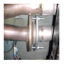
INSTALL PASS. SIDE HEADPIPE # A USING HARDWARE # H. DO NOT TIGHTEN. INSERT HANGER INTO RUBBER GROMMET, NEXT SLIP DR. SIDE HEADPIPE # B ONTO FACTORY PIPE USE CLAMP # F TO SECURE. DO NOT TIGHTEN.
