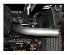
SLIDE TAILPIPE #D INTO MUFFLER 1-1/2" TO 2". INSERT WELDED HANGER INTO RUBBER GROMMET AND ATTACH TO HANGER # G.
