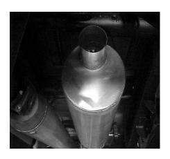
INSTALL MUFFLER # C ONTO HEADPIPES 1 ½"-2". USE CLAMPS # G TO SECURE OUTLET OF MUFFLER, IT SHOULD BE AT THE 12 O'CLOCK POSITION. USE A JACKSTAND TO SUPPORT MUFFLER.
