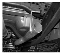
INSTALL HEADPIPE #A ONTO STOCK FLANGE USING THE FACTORY BOLT TO SECURE IT. DO NOT TIGHTEN. NEXT INSTALL HEADPIPE #B ONTO #A HEADPIPE YOU WILL USE CLAMP #F TO SECURE HEADPIPE #A TO #B, DO NOT TIGHTEN. INSERT WELDED HANGER INTO RUBBER GROMMET.
