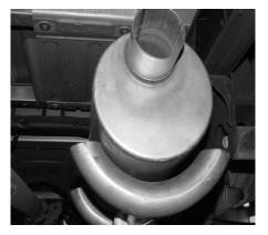
INSTALL MUFFLER #C ONTO HEADPIPE. OUTLET SHOULD BE AT THE 11 O'CLOCK POSITION. USE CLAMP #F TO SECURE MUFFLER TO THE HEADPIPE, DO NOT TIGHTEN. USE A JACK STAND TO SUPPORT MUFFLER. INLET OF MUFFLER IS LOOKING INTO LOUVERS.
