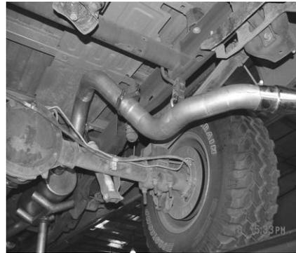
INSTALL OVERAXLE TAILPIPE #C INTO THE OUTLET OF THE MUFFLER 1 1/2" TO 2" USING CLAMP #E TO SECURE PIPE TO MUFFLER. INSERT WELDED HANGER INTO RUBBER GROMMET.
