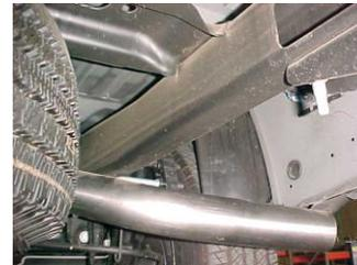
Install over axle tailpipe #C into muffler 1 1/2" to 2". Secure together with clamp #C. Do not tighten. Insert hanger into rubber grommet.
