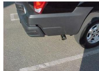
Install stainless steel tip. Clamp down. When you have everything in place, firmly tighten all bolts and clamp down securely. To clean stainless steel tip use any stainless steel cleaner and a scotch brite pad.
