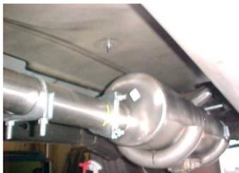
Install muffler #B onto head pipe 1-1/2" to 2" with the louvers facing towards the converter. Use a jack stand to support the muffler. Use clamp #E to secure the muffler to the head pipe. Do not tighten. Muffler inlet is looking into the louvers. Outlet should be at 10 o'clock position.
