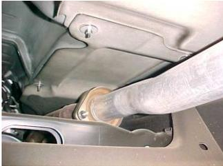
Lay out the exhaust on the floor so it looks like the drawing and compare parts with manual. To remove the stock exhaust remove it from the 2-bolt flange located behind the muffler cut your tailpipe off for easier removal. Leave all rubber grommets in place. Use WD-40 to aid in the removal of exhaust and hanger. **Do not discard stock hardware, you will reuse it.**
