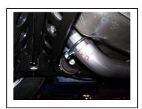
Install muffler # D onto the tailpipe.
