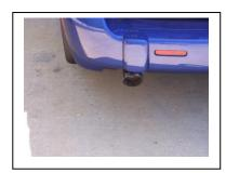
Install stainless steel tip. Clamp down. When you have everything in place, firmly tighten all bolts and clamps down securely. To clean stainless steel tip use any stainless steel cleaner and Scotch Brite pad.
