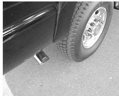
WELD PASSENGER INLET OF THE MUFFLER TO THE FACTORY HEADPIPE. THEN TIGHTEN ALL CLAMPS AND HANGERS. INSTALL YOUR STAINLESS STEEL TIP. USE ANY ALUMINUM OR STAINLESS STEEL CLEANER TO POLISH YOUR TIP.
