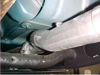
Lay out the exhaust on the floor so it looks like the drawing and compare parts with manual. To remove the stock exhaust Remove it from the stock 2-bolt flange located just behind your catalytic converter. Leave all rubber grommets in place. Use WD-40 to aid in removal of exhaust and hangers. Do not discard your factory hardware. **You will re-use your stock bolts.**
