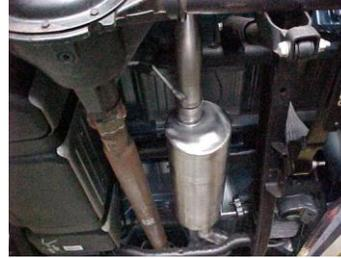
Install the over axle tailpipe #C into the muffler 1-1/2" to 2". Secure to the muffler using clamp # F. Do not tighten.
