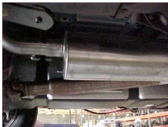
Install muffler onto head pipe 1-1/2" to 2" with the louvers facing towards the converter. Use a jack stand to support the muffler. Use clamp #F to secure the muffler to the head pipe. Do not tighten. Muffler inlet is looking into the louvers. Outlet should be at the 11 o'clock position.
