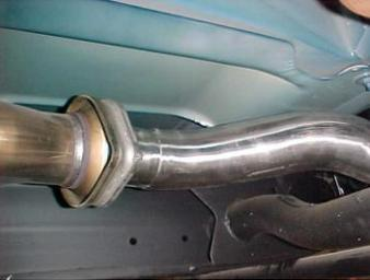
Install head pipe #A on to your existing stock 2-bolt flange using your factory hardware. Use a jack stand to support the converter. Insert welded hanger into rubber grommet. Do not tighten.
