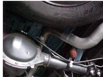
Insert welded hanger into rubber grommet.
