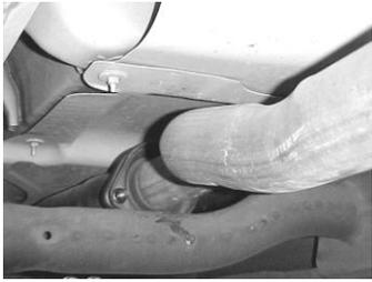
Lay out the exhaust on the floor so it looks like the drawing and compare parts with manual. To remove the stock exhaust, remove it from the factory 2-bolt flange located in front of the muffler. **Do not discard the factory hardware you will re-use them.** Leave all rubber grommets in place. Use WD-40 to aid in removal of exhaust and hangers. Cut off your
