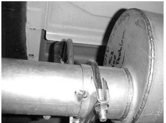
Install muffler onto head pipe 1-1/2" to 2" with the louvers facing towards the converter. Use a jack stand to support the muffler. Use clamp #G to secure the muffler to the head pipe. Insert hanger into rubber grommet. Do not tighten. Muffler inlet is looking into the louvers.
