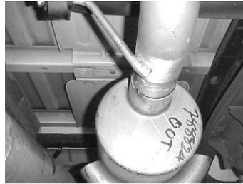
Install the tailpipe # C into the muffler at least 1-1/2" to 2". Secure pipe to the muffler using clamp # E. Do not tighten. Insert welded hanger into rubber grommet.
