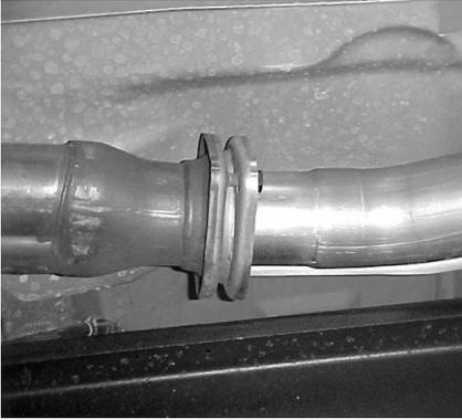
TO REMOVE STOCK EXHAUST UNBOLT THE STOCK EXHAUST AT THE FLANGE BEHIND THE Y-PIPE AND REMOVE. MAKE SURE TO LEAVE ALL RUBBER GROMMETS IN THE FACTORY LOCATION. **YOU WILL RE-USE STOCK NUTS AND BOLTS.** FOR EASIER REMOVAL OF EXHAUST, CUT BEHIND THE MUFFLER. USE WD-40 TO REMOVE HANGERS FROM GROMMETS.
