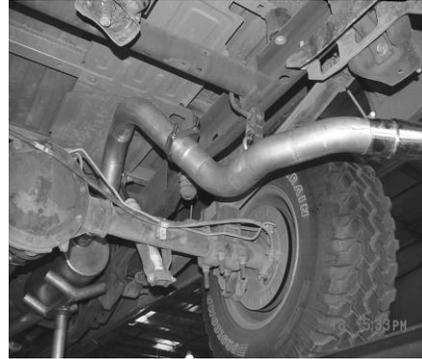
INSTALL OVERAXLE TAILPIPE #C TO THE OUTLET OF THE MUFFLER USING CLAMP #E. INSERT WELDED HANGER INTO RUBBER GROMMET.
