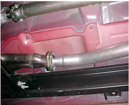
BOLT HEADPIPE #A TO THE STOCK FLANGE RE-USING THE FACTORY NUTS & BOLTS. INSERT WELDED HANGER INTO RUBBER GROMMET.
