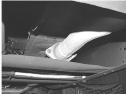
TO REMOVE STOCK EXHAUST- UNBOLT IT FROM THE TWO-BOLT FLANGE LOCATED BEHIND THE STOCK CATALYTIC CONVERTER.
