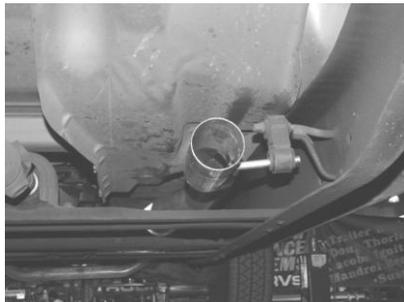
BOLT HEADPIPE #A ONTO STOCK FLANGE RE-USING FACTORY GASKETS AND BOLTS AND GASKET # G. INSERT WELDED HANGER INTO RUBBER GROMMET. DO NOT TIGHTEN. USE CLAMP #F TO SECURE MUFFLER TO HEADPIPE. DO NOT TIGHTEN.
