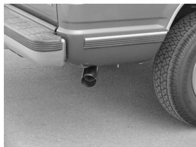
INSTALL STAINLESS TIP. USE ANY ALUMINUM OR STAINLESS CLEANER TO POLISH YOUR TIP. TIGHTEN ALL NUTS, BOLTS & CLAMPS.
