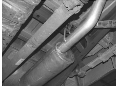
SLIDE OVERAXLE TAILPIPE #C INTO MUFFLER AT LEAST 1"-2". THE TAILPIPE END THAT GOES INTO THE OUTLET OF THE MUFFLER HAS THE LONGEST WELDED HANGER. SLIDE WELDED HANGERS INTO RUBBER GROMMETS. USE CLAMP # F TO SECURE PIPE TO MUFFLER. DO NOT TIGHTEN.
