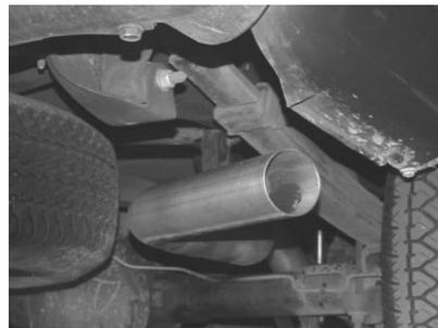
SLIDE MUFFLER # B ONTO HEADPIPE AT LEAST 1"-2" WITH INLET TOWARDS THE MOTOR. OUTLET SHOULD BE AT 9 O'CLOCK POSITION. INLET OF MUFFLER IS LOOKING INTO THE LOUVERS. USE A JACKSTAND TO SUPPORT THE MUFFLER.
