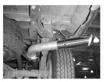
INSTALL EXIT PIPE #E. USE CLAMP #H TO CLAMP IT DOWN. DO NOT TIGHTEN. ROTATE THE PIPE'S UNTIL YOU HAVE A MINIMUM OF A 1" CLEARANCE ON ALL PIPE'S AND HANGERS FROM ALL RUBBER BRAKE LINE'S, TIRES, SHOCKS, FUEL LINES, ETC. THEN TIGHTEN ALL CLAMPS AND HANGERS.
