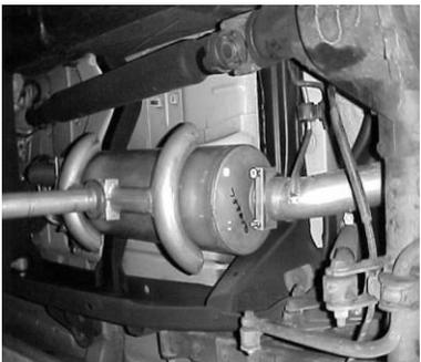
SLIDE MUFFLER WITH DUAL INLET ONTO HEADPIPE AT LEAST 1-1/2" TO 2". MUFFLER OUTLET SHOULD BE AT THE 12 O'CLOCK POSITION. USE CLAMPS #F TO ATTACH HEADPIPE. MAKE SURE INLETS AND MUFFLER IS LEVEL. AND TIGHTEN DOWN. USE JACK STAND TO SUPPORT MUFFLER.
