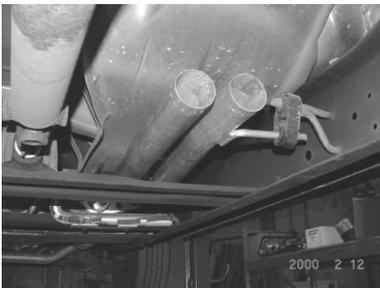
BOLT HEADPIPE #A USING SUPPLIED FLANGE GASKET AND REUSING FACTORY BOLTS. APPLY A SMALL A MOUNT OF HIGH-TEMP O2 SENSOR SAFE SILICONE ON THE FLANGE TO PREVENT ANY LEAKS. INSERT WELDED HANGER INTO RUBBER GROMMET. DO NOT TIGHTEN
