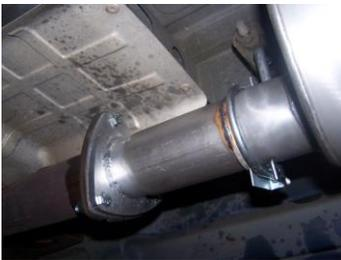
BOLT FRONT HEADPIPE #A ONTO STOCK FLANGE USING SUPPLIED BOLT KIT #H AND GASKET #I. INSERT WELDED HANGER INTO RUBBER GROMMET.
