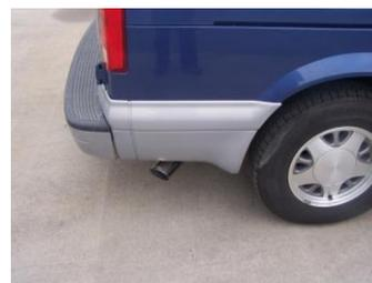
INSTALL STAINLESS STEEL TIP, CLAMP DOWN. NOW TIGHTEN ALL BOLTS AND CLAMPS. TO CLEAN TIP USE SCOTCH BRITE AND ANY STAINLESS OR ALUMINIUM CLEANER.
