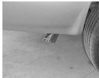
Install stainless steel tip. Clamp down. To clean stainless steel tip, use a scotch brite pad and any stainless steel or aluminum cleaner. When you have everything in place, firmly tighten all bolts and clamp down securely.
