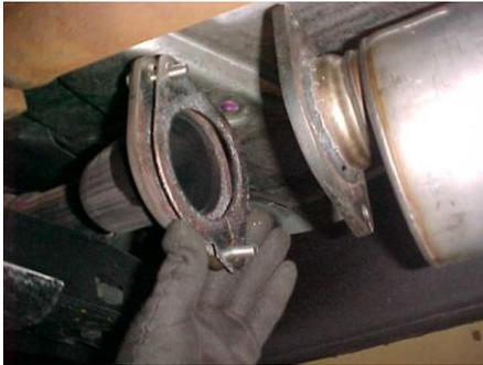
Lay out the GIBSON EXHAUST SYSTEM on the floor so it looks like the drawing and match the part numbers with the parts list. (Note: Drawing is not exact except for placement of parts only!) Raise vehicle and support with stands. Unbolt stock exhaust in front of your stock muffler. Use jackstands to support the converter so it won't drop. Leave all rubber mounting grommets in place.
