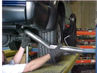
Install the overaxle tailpipe #B. Attach to muffler with hanger #D, Insert welded hanger into factory rubber grommet.
