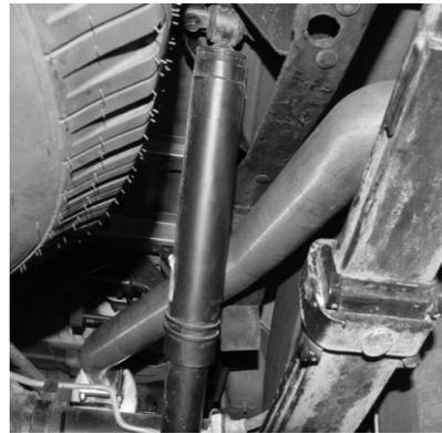
INSTALL TAILPIPE #C ONTO MUFFLER 1-1/2" TO 2". THE TAILPIPE WILL GO BETWEEN TIRE AND SHOCK, INSTALL FROM THE REAR OF THE VEHICLE. INSERT WELDED HANGER INTO THE RUBBER GROMMET. AND ATTACH WITH HANGER # E.
