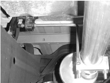
INSTALL MUFFLER #B ONTO HEADPIPE 1-1/2" TO 2" WITH INLET TOWARDS THE ENGINE. OUTLET SHOULD BE AT THE 2 O'CLOCK POSITION. USE CLAMP #E AND #F TO SECURE MUFFLER TO THE HEADPIPE, INSERT MUFFLER HANGER INTO RUBBER GROMMET. DO NOT TIGHTEN. THE INLET OF THE MUFFLER IS LOOKING INTO THE
