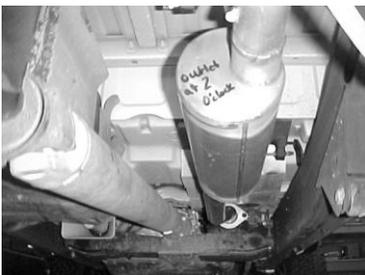
INSTALL REAR MUFFLER HANGER #E INTO RUBBER GROMMET. THE CLAMP WILL BE USED TO SECURE THE TAILPIPE TO THE MUFFLER, DO NOT TIGHTEN.
