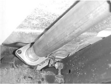
TO REMOVE STOCK EXHAUST UN-BOLT IT FROM THE 2-BOLT FLANGE LOCATED BETWEEN THE CATALYTIC CONVERTER AND THE MUFFLER. NOW CUT OFF YOUR STOCK TAILPIPE JUST BEHIND THE MUFFLER AND REMOVE. LEAVE ALL RUBBER GROMMETS ON THE HANGER. USE WD-40 TO AID IN REMOVAL OF EXHAUST AND HANGERS. INSTALL HEADPIPE #A, USE # G GASKET, AND RE-USE YOUR FACTORY BOLTS. INSERT WELDED HANGER INTO RUBBER GROMMET. DO NOT TIGHTEN.
