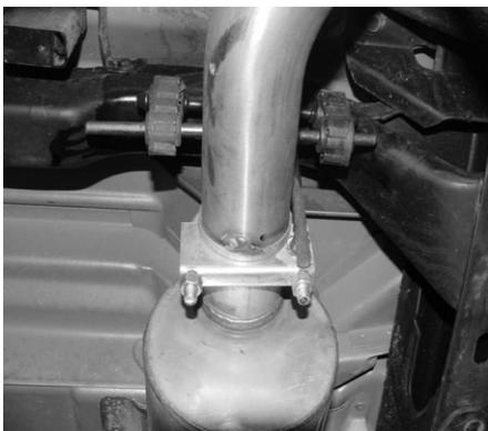
INSTALL REAR MUFFLER HANGER #E INTO RUBBER GROMMETS, LONGER SIDE OF THE HANGER WILL GO TOWARDS THE DRIVERS SIDE. THE CLAMP WILL BE USED TO SECURE THE TAILPIPE TO THE MUFFLER, DO NOT TIGHTEN.
