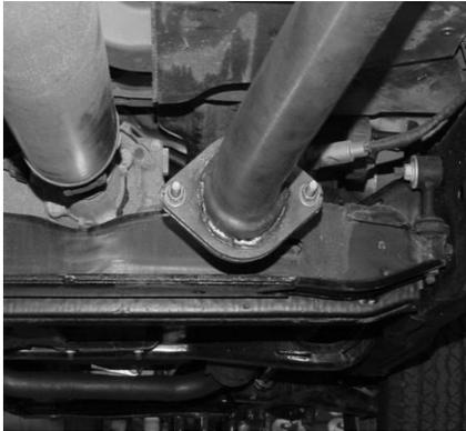
TO REMOVE STOCK EXHAUST UN-BOLT IT FROM THE 2-BOLT FLANGE LOCATED BETWEEN THE CATALYTIC CONVERTER AND THE MUFFLER. NOW CUT OFF YOUR STOCK TAILPIPE JUST BEHIND THE MUFFLER AND REMOVE. LEAVE ALL RUBBER GROMMETS ON THE HANGER. USE WD-40 TO AID IN REMOVAL OF EXHAUST AND HANGERS. INSTALL HEADPIPE #A, USE #G GASKET, NUTS AND BOLTS, KIT # H. INSERT WELDED HANGER INTO RUBBER GROMMET. DO NOT TIGHTEN.
