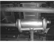
Lay out the GIBSON EXHAUST SYSTEM on the floor so it looks like the drawing. Match all part numbers with the manual. Unbolt stock flange from behind the catalytic converter. Leave all rubber grommets in place.Use jack stands to support converter.
