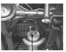
Install muffler 1-1/2" to 2" onto the front headpipe with louvers in muffler facing towards the converter and clamp down using #F. Use a jack stand to support the muffler. Outlet of muffler should be clocked at 12 o'clock. Muffler inlet is looking into the louvers. Install rear hanger #G onto muffler and insert into rubber grommet. Bolts will face the driverside. Do not tighten
