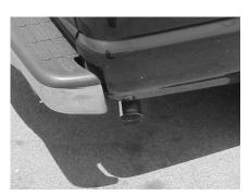
Install stainless steel tip. Clamp down. To clean stainless steel tip use any stainless or aluminum cleaner. When you have everything in place, tighten all bolts, flange and clamps.
