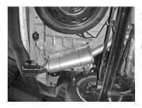
INSTALL MUFFLER ASSEMBLY #C. SLIP THE WELDED HANGER INTO THE FACTORY RUBBER GROMMETS. RE-CONNECT THE GROUND STRAP TO THE MUFFLER ASSEMBLY USING BOLT KIT #F.
