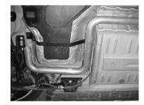
SLIP FRONT EXTENSION PIPE #B INTO THE OUTLET OF THE RESONATOR. USE CLAMP #D TO ATTACH THE EXTENSION PIPE TO THE RESONATOR. INSTALL REAR PIPE #E TO FRONTPIPE #B. SLIP THE WELDED HANGER INTO THE FACTORY RUBBER GROMMET AND ATTACH WITH CLAMP #D.
