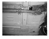
REMOVE THE FRONT EXTENSION PIPE BY DISCONNECTING THE EXHAUST BEHIND THE CONVERTER. LEAVE ALL FACTORY RUBBER GROMMETS IN PLACE YOU MAY NEED TO HEAT UP THE EXTENSION PIPE TO REMOVE.
