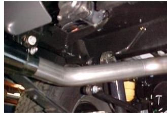
5. Slide the second driver side over axle tailpipe #C onto pipe #B 1.5-2". Secure pipes using clamp #F. Do not tighten. Insert welded hanger into rubber grommet.
