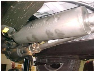
3. Slide muffler #A onto headpipe 1½"-2". Use a jack stand to support the muffler. Make sure muffler outlets are level. Use clamp #G to secure the muffler to the headpipe. Do not tighten.
