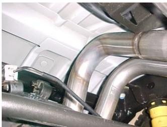
4. Slide driver side over axle tailpipe #B into muffler 1.5-2". Use clamp #F to secure tailpipe to muffler. Do not tighten. Insert welded hanger into rubber grommet.
