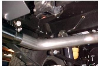
6. Slide the second driver side over axle tailpipe onto the first 1.5-2". Secure pipes using clamp #G. Do not tighten. Insert welded hanger into rubber grommet.
