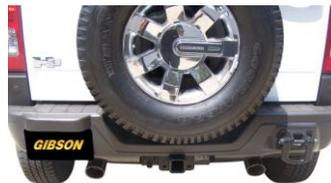
8. Install stainless steel tip. Clamp down. When you have everything in place, firmly tighten all bolts and clamps down securely. Use stainless steel cleaner and a Scotch Brite pad weekly to prevent tip from discoloration. Inspect all fasteners after 25-50 miles of operation and re-tighten as necessary.
