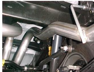
5. Slide the passenger side tailpipe #E into muffler 1.5-2". Insert welded hanger into rubber grommet. Use clamp #G to secure tailpipe to muffler. DO NOT TIGHTEN.
