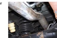
5. Slide the over axle tailpipe #C into the muffler 1.5-2". Use clamp #E to secure tailpipe to muffler. Do not tighten. Insert welded hangers into rubber grommets.
