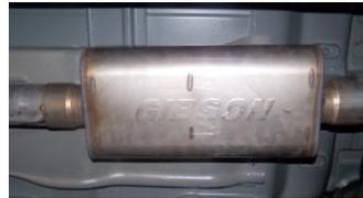
4. Slide muffler #B onto headpipe 1.5-2". Use a jack stand to support the muffler. Use clamp #E to secure the muffler to the headpipe. Do not tighten.
