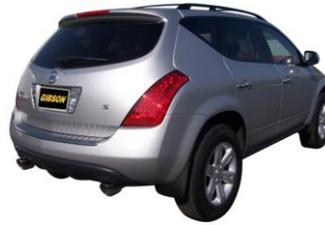
8. Install stainless steel tips. Clamp down. When you have everything in place, firmly tighten all bolts and clamps down securely. Use stainless steel cleaner and a Scotch Brite pad weekly to prevent tip from discoloration. Inspect all fasteners after 25-50 miles of operation and re-tighten as necessary.
