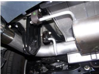
3. Install muffler assembly onto factory pipe. Insert hangers into rubber grommets. Use clamp #B to secure pipes together. Do not tighten.
