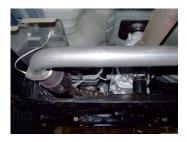
3. Install headpipe #A onto the existing stock flange and attach with the factory nuts. Re-attach the ground strap. Do not tighten the nuts.
