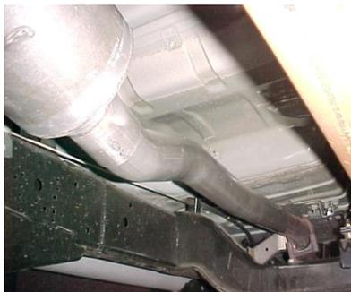
SLIDE HEADPIPE # A ONTO YOUR FACTORY PIPE 1-1/2" TO 2". USE CLAMP # F TO SECURE. DO NOT TIGHTEN.
