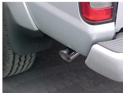
NEXT INSTALL YOUR STAINLESS STEEL TIP TO YOUR DESIRED LOOK. USE A STAINLESS OR ALUMINUM CLEANER TO POLISH TIP. NOW TIGHTEN ALL CLAMPS STARTING FROM THE FRONT AND WORKING BACK.
