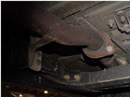
REMOVE THE STOCK EXHAUST BY UNBOLTING THE 17MM BOLTS IN FRONT OF THE MUFFLER. YOU WILL RE-USE YOUR FLANGE BOLTS. DO NOT DAMAGE THE FACTORY GASKET YOU WILL NEED TO RE-USE! THEN CUT DIRECTLY BEHIND THE MUFFLER AND REMOVE THE STOCK EXHAUST.
