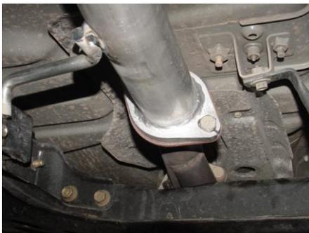
INSTALL THE HEADPIPE RE-USING THE FACTORY GASKET AND BOLTS. APPLY A SMALL AMOUNT OF HI-TEMP GASKET SEALER ONTO THE GASKET TO ENSURE A LEAK FREE CONNECTION. DO NOT TIGHTEN. INSTALL HEADPIPE HANGER USING ONE OF THE FACTORY NUTS AND BOLT #F.
