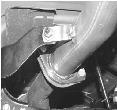
REMOVE THE STOCK EXHAUST BY UNBOLTING THE 17MM BOLTS IN FRONT OF THE MUFFLER. UN-BOLT FACTORY HEADPIPE (YOU WILL RE-USE YOUR FLANGE BOLTS). DO NOT DAMAGE THE FACTORY GASKET YOU WILL NEED TO RE-USE! THEN CUT DIRECTLY BEHIND THE MUFFLER AND REMOVE THE STOCK EXHAUST.
