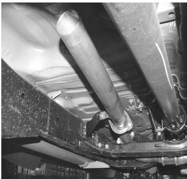
INSTALL THE HEADPIPE RE-USING THE FACTORY GASKET AND BOLTS. APPLY A SMALL AMOUNT OF HI-TEMP GASKET SEALER ONTO THE GASKET TO ENSURE A LEAK FREE CONNECTION. DO NOT TIGHTEN.
