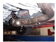
2.Remove the whole exhaust from the clamps (located just after your factory headers). To make it easier, remove the support in the *middle* of the car. Do Not Disgard. You will reinstall.
