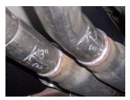
2. To remove stock exhaust, remove from clamps located just after the catalytic converter do not damage or remove the rubber grommets as you well re-use them to mount your new system.
