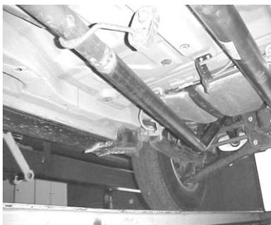
INSTALL FRONT EXTENSION PIPE #F TO HEADPIPE AND USE CLAMP #E. INSTALL THE RESONATOR #A AND ATTACH TO EXTENSION PIPE WITH CLAMP #E. THE INLET OF THE RESONATOR IS LOOKING INTO THE LOUVERS. USE A JACK STAND TO SUPPORT THE RESONATOR.
