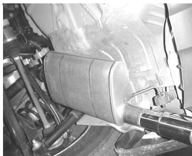
SLIP THE MUFFLER ASSEMBLY # C ONTO THE REAR EXTENSION PIPE. INSERT THE WELDED HANGER INTO THE RUBBER GROMMET AND ATTACH TO PIPE WITH CLAMP #F. ROTATE ALL PIPES UNTIL YOU HAVE A MINIMUM OF A 1-1/2" CLEARANCE FROM ALL RUBBER BRAKE LINE'S, TIRES, SHOCKS, ETC.
