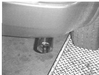
INSTALL YOUR STAINLESS STEEL TIP. USE ANY ALUMINUM OR STAINLESS STEEL CLEANER TO POLISH YOUR TIP. TIGHTEN ALL CLAMPS AND HANGERS.
