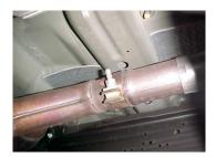
REMOVE YOUR STOCK **EXHAUST FROM THE** CLAMP LOCATED JUST AFTER YOUR STOCK Y-PIPE. CUT OFF TAILPIPE JUST BEHIND THE MUFFLER USE WD-40 TO AID IN REMOVAL OF HANGER LEAVE RUBBER GROMMETS IN PLACE. NEXT, INSTALL HEADPIPE #A ONTO Y-PIPE USING CLAMP #F TO SECURE, DO NOT TIGHTEN.
