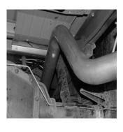
INSTALL OVERAXLE TAILPIPE #C INTO THE MUFFLER NO MORE THAN 1 ½" TO 2". INSERT WELDED HANGER INTO RUBBER GROMMET. ATTACH USING CLAMP # G.
