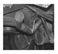
INSTALL TURNOUT PIPE #D TO THE OVERAXLE TAILPIPE. ROTATE PIPE SO IT IS AT THE CORRECT ANGLE FOR YOUR VEHICLE. USE CLAMP #G TO ATTACH.
